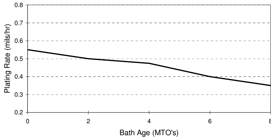
Plating Rate vs. Bath Age pH - 4.8 / 190 deg. F
